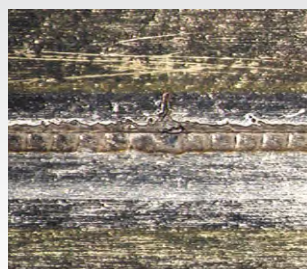
Contamination caused by tin splash detected by SWM-2.
