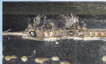
Welding defect due to overlacquering detected by OCR-R.
