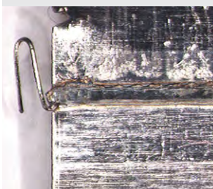
Cutting defect at trailing end detected by SWM-2.
