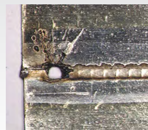
Overlacquering about 3 mm before trailing end detected by SWM-2.
