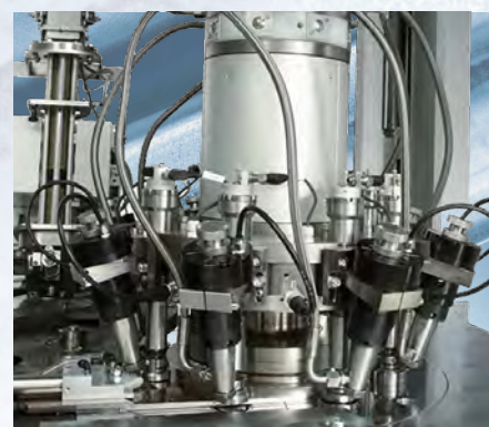
Circular compound distribution system
